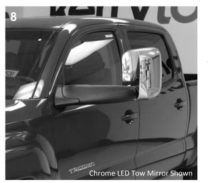
8. Bolt the new tow mirror on and reconnect plug. Use the reverse steps above to finish installation. RH mirror installation will be performed in the same manner. For Plug & Play tow mirrors, the installation manual stops here.
